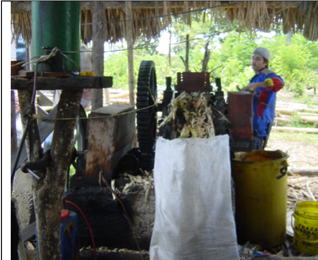
Photo 1: Fractionating sugar cane stalks into sugar-rich juice and residual fibre (Bagasse) (Source: T R Preston, unpublished data)
