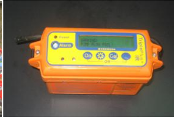
Photo 2. Measurement of percentage of methane with the Crowcon meter
