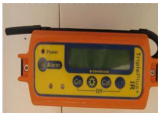
Photo 2. Measurement of percentage of methane with the Crowcom meter
