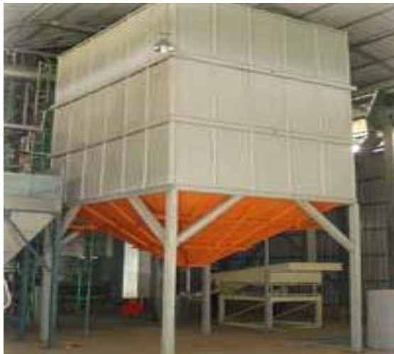
Photo 3: Dryer machine utilizing rice husk as feedstock
