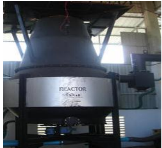
Photo 4: Downdraft gasifier, designed for rice husk feedstock
