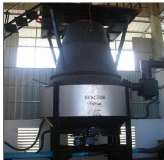
Photo 2: Rice husk gasifier at rice milling station
