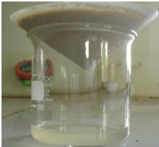
Photo 12: Adding water to saturate the soil then allowing the water to drain for 24 hours to determine water holding capacity
