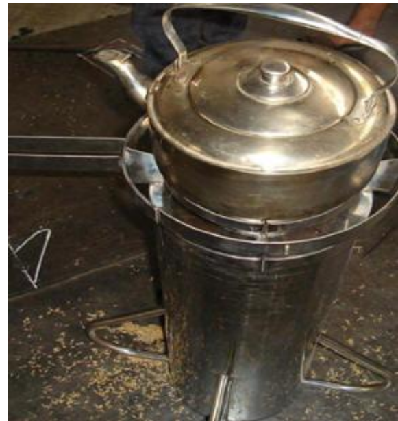
Photo 3: Gasifier stove from top view (Olivier 2010) Photo 4: Gasifier stove, boiling water (Olivier 2010)
