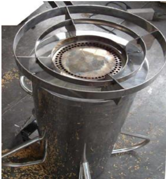
Photo 3: Gasifier stove from top view (Olivier 2010) Photo 4: Gasifier stove, boiling water (Olivier 2010)
