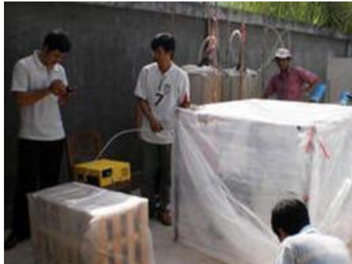
Photo 3. Goats were confined in a closed space for the measurement of the eructed gases with the Gaset 4030 equipment
