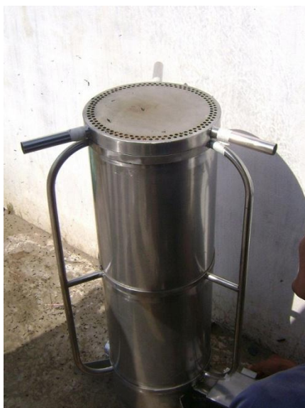
Photo 4: The updraft gasifier stove
