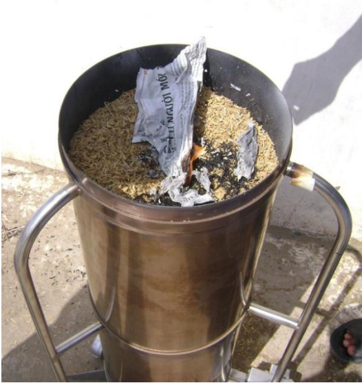
Photo 4: The updraft TLUD gasifier stove
