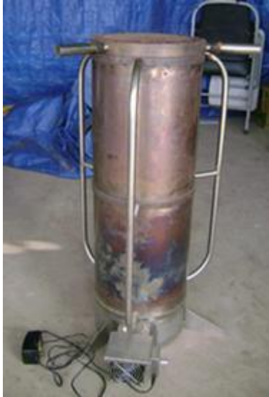
Photo 4: The updraft TLUD gasifier stove
