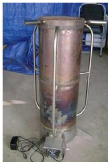
Photo 10: The updraft gasifier stove
