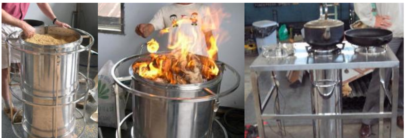
Photos 1-3: The TLUD gasifier stove developed in Vietnam (Olivier 2010)
