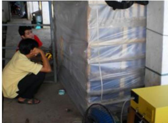
Photo 5. Wooden crates enclosed in plastic used to house the cattle during the 5 minute period of adaptation/measurement using the GASMET infra-red analyser.
