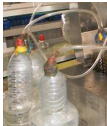
Photo 2. Using "plasticine" to seal the junction between the gas inlet tube and the bottle used to measure gas volume by water displacement
