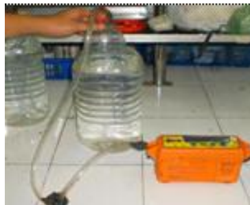
Photo 3. Measurement of methane with the Crowcom meter
