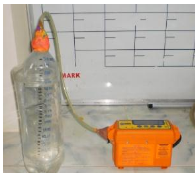
Photo 3. Measurement of methane with the Crowcom meter
