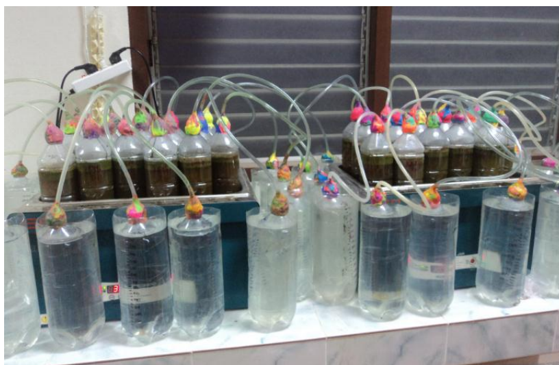
Photo 1. The in vitro fermentation system using recycled water bottles and water displacement to measure gas production
